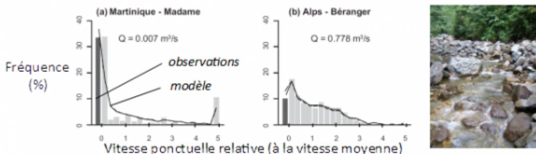
Examples of statistical hydraulic models (Girard et al. 2014) predicting velocity distributions in stream reaches of different rivers. The approach is particularly relevant in very complex flows (tropics, mountains). The input variables of statistical models are simple to measure, which facilitates their use for studies at the scale of the reaches as well as at the scale of the watersheds.
